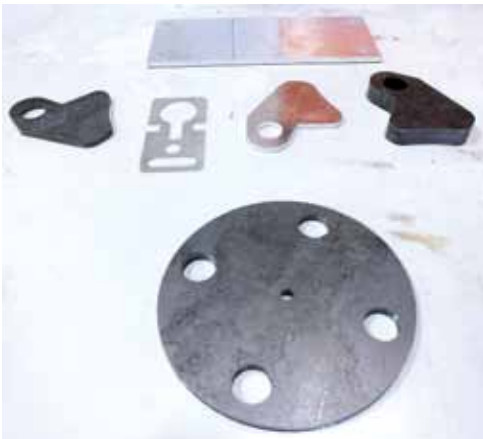
Samples of parts cut on Baseline's Ferric-Ermaskan Fibermak fiber laser cutting system.
