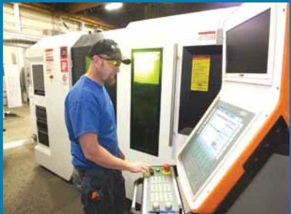
Machine operator Les McCrory adjusts parameters for a part in the fiber laser cutting machine.
