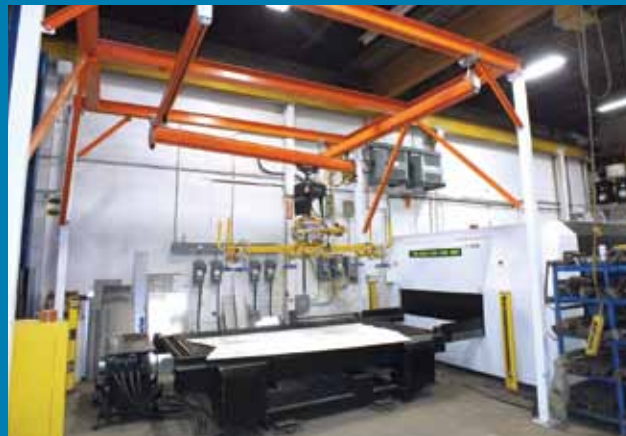
Baseline designed its own sheet loading system for the fiber laser system and plans to market it to other laser cutting shops.
